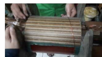
Gambar 14. Pemasangan Oil Duct
